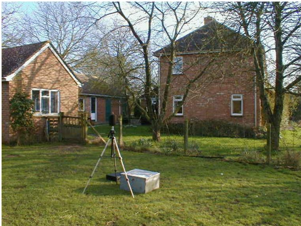
Figure 7: Typical Long-Term Noise Monitoring Setup
